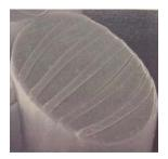
WRAMP fiber is a bicomponent fiber with a stacked structure consisting of eleven alternating layers or "stripes" of polyester and nylon. Mild refining of this fiber causes it to split into approximately 0.3 micro denier ribbon shaped fibers. Papers made from WRAMP fiber, or blends with wood pulp, exhibit very high tear factor, low air permeability, smaller pore size, high luster, good printability and high fold endurance.
